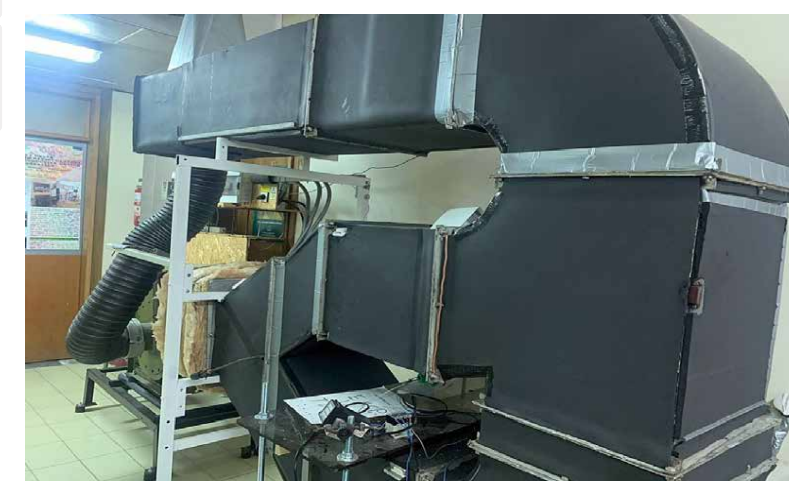
Fig 3. Photo of experimental convective dryer
